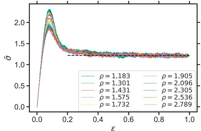
FIG. 6. Reduced stress-strain curves along isomorph determined by the procedure illustrated in Fig. 5. Glasses cooled (at lowest density) at rate  $R_{c,0} = 10^{-5}$  and sheared at reduced strain rate  $\dot{\epsilon} = 10^{-3}$ .
