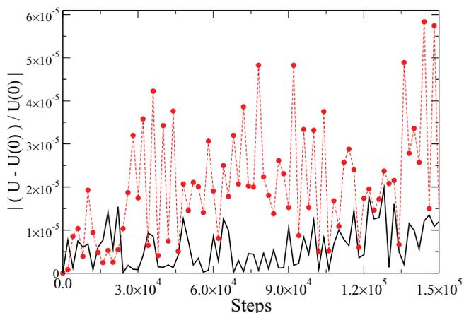
FIG. 2. Evolution of  $|(U - U(0))/U(0)|$  for a simulation using the basic *NVU* algorithm. The red curve gives results from a simulation where the potential is cut and shifted at  $r = 2.5\sigma$ , the black curve gives results for a smoothed force potential.
