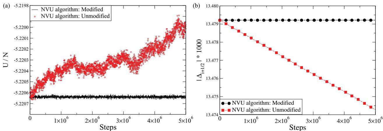
FIG. 3. (a) Evolution of  $U$  with and without the numerical stabilization (Eq. (20)): The red curve gives results using the basic *NVU* algorithm Eq. (17) with two identical initial potential energies and smoothed force potential. The black curve gives simulation results under the same conditions using the final *NVU* algorithm (Eq. (20)). (b) Evolution of the step length for the same simulations.
