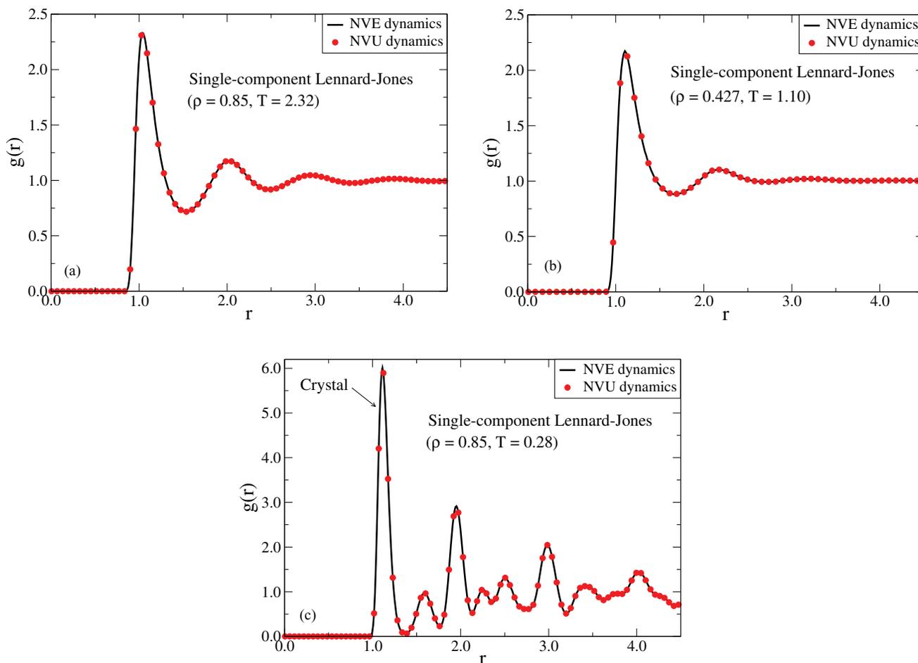
FIG. 5. Radial distribution functions  $g(r)$  for a single-component Lennard-Jones system at the following state points: (a)  $T = 2.32$  and  $\rho = 0.85$ ; (b)  $T = 1.10$  and  $\rho = 0.427$ ; (c) the crystal at  $T = 0.28$  and  $\rho = 0.85$ . The black curves show results from *NVE* simulations, the red dots show results from *NVU* simulations (Eq. (20)).
