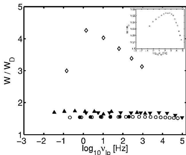
FIG. 12. Dielectric data. Loss peak width ( $W/W_D$ ) of the dielectric relaxation curve based on  $-\epsilon''$ , (see Fig. 11 for details). No such data exist for squalane and PB20 as their data are too noisy due to their small dielectric relaxation strength. The inset shows the same data for TPG with a different scaling. TPE ( $\blacktriangle$ ), DC704 ( $\blacktriangledown$ ), PPE ( $\bullet$ ), DHIQ ( $\diamond$ ), and TPG ( $\circ$ ).
