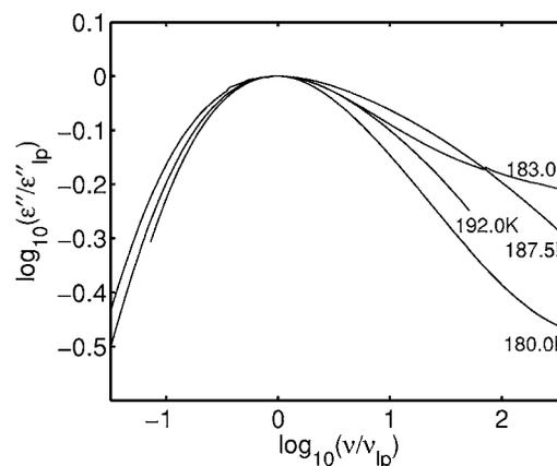
FIG. 14. Dielectric loss of DHIQ scaled by the maximum loss and the loss peak frequency (note the scale of the axis, the beta peak is outside the zoom). It is seen that the alpha peak broadens upon cooling as the beta peak emerges, while it gets narrower again as the beta peak separates from the alpha peak.
