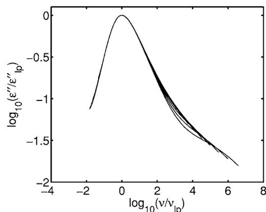
FIG. 13. Dielectric loss of TPG scaled by the max loss and the loss peak frequency. The temperatures shown are 196.0–212.0 K in steps of 2 K. There is a spreading of the curves at the high-frequency side where the Johari-Goldstein beta peak appears, while the alpha peaks appear to collapse on a single master curve.
