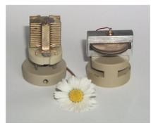
Dielectric: 22-layer gold platen capacitor with empty capacitance of 68 pF.  $10^{-3} - 10^6$  Hz
